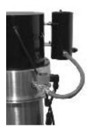
Accumulator blowback with large solenoid assures maximum filter cleaning of dual bag filter assembly.
