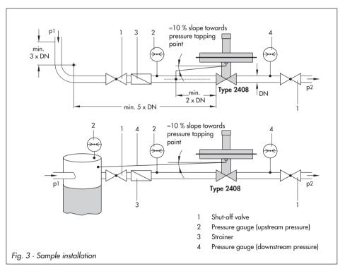
When tapping the pressure at a straight pipeline section, observe a minimum distance of at least twice the nominal valve size to the regulator.
