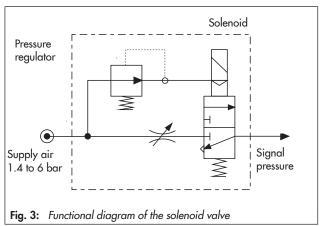
When the integrated solenoid valve is energized, supply air is applied to the actuator. The speed of air supply is adjustable at a restriction. When the solenoid valve is de-energized, the actuator is vented and the control valve moves to its fail-safe position.
