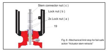
The mechanical limit stop for the actuator fail-safe action Air-toclose is made by two hexagon nuts ( a ), which are mounted outside on the valve stem.
