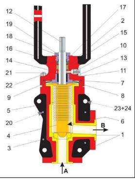
Fig. 2 - Cross-section through a Series 8a Angle Valve => see Table 1 for list of parts
